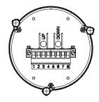
Standard NORIMETER 3 indicators have an 8-pole connector with 4 connection options that are completely galvanically isolated from one another:
